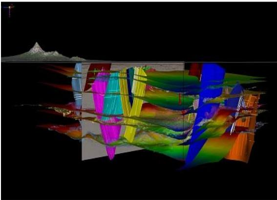
*2D and 3D seismic data, structural interpretation and model in one integrated display in the 3D Canvas*
