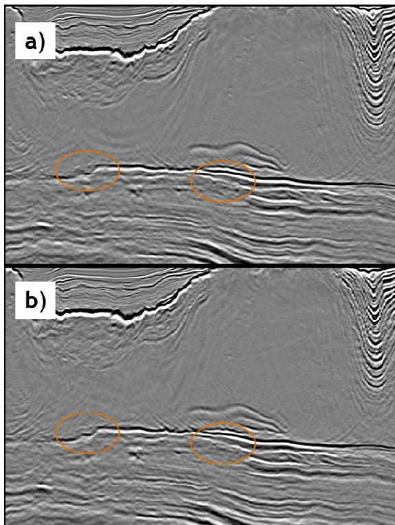
Figure 5: Seismic amplitude migrated with different velocity models: (a) tomography-only and (b) salt inversion. The orange ellipses highlight the base of salt and the reflector continuity.
