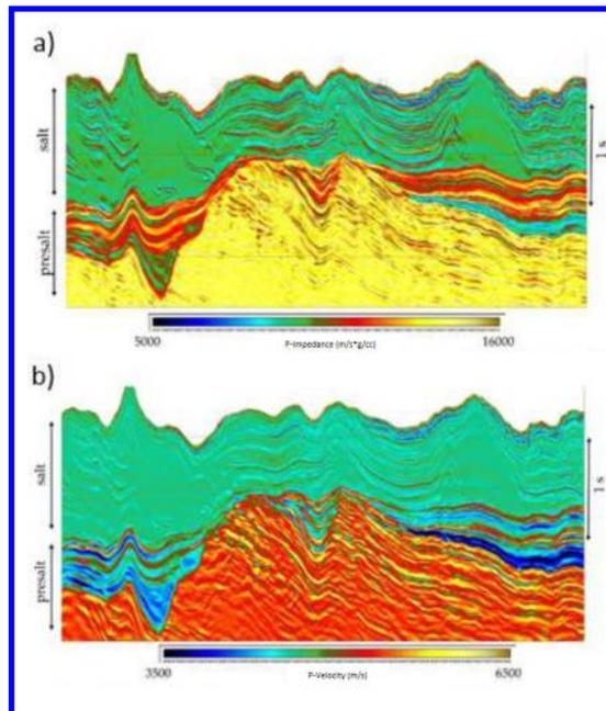
Figure 3: (a) P-Impedance of the Salt Section and the Pre-Salt Section and (b) generated compressional velocity after applying the cross-plot rules on the P-impedance volumes. (adapted from Fonseca *et al.*, 2018).
