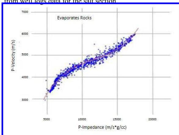
Figure 2: Relation between compressional velocity and acoustic impedance for Evaporates Rocks (adapted from Fonseca *et al.*, 2018).
