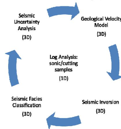
Figure 1: Proposed workflow to generate a more realistic seismic velocity model (adapted from Maul *et al.*, 2016 in González *et al.*, 2016).
