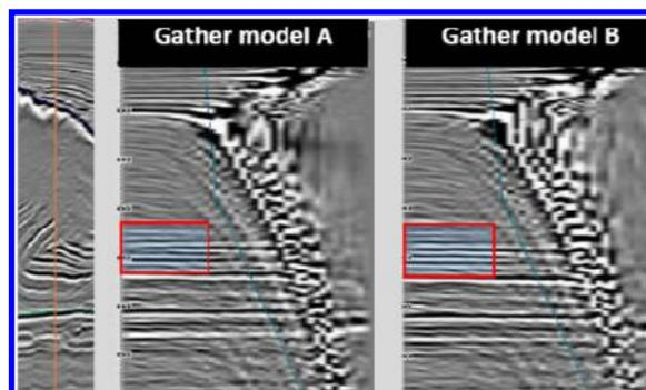
Figure 4: Subset of a migrated amplitude section. The orange line represents the trace whose depth migrated gathers are displayed. The letters refer to the velocity model: (A) Previous velocity model from tomography and (B) updated velocity model with the salt region modelled through impedance. The red boxes highlight stratification events, demonstrating an enhancement of such events within the salt section. (Adapted from Fonseca *et al.*, 2017 in Fonseca *et al.*, 2018).
