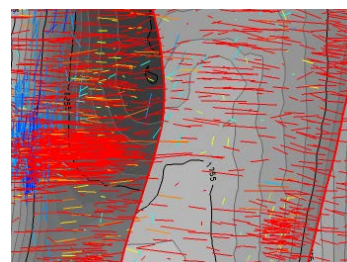
Sh,max after 25 years of production is displayed in SKUA-GOCAD. Stresses are locally reoriented in the fault neighborhood.
