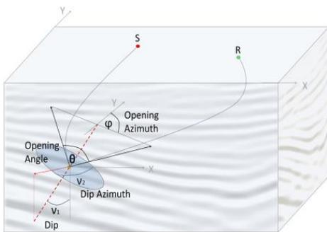
Figure 1. Example of a specular ray pair used in tomography
