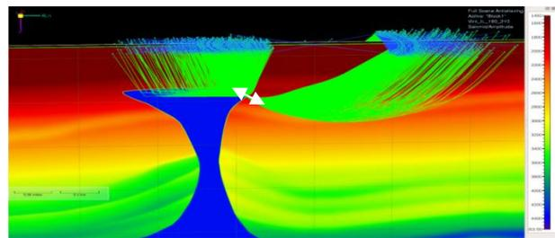
Figure 4. Inward and outward specular ray pairs from the same subsurface point (BP TTI synthetic salt model)
