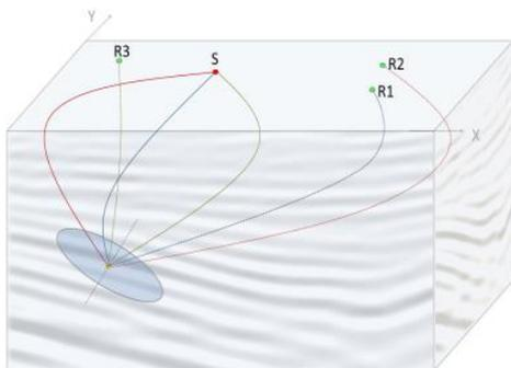
Figure 3. Three specular ray pairs showing shot domain multi-pathing. Their corresponding seismic event will be mapped into the same bin in the I-OVT gather.
