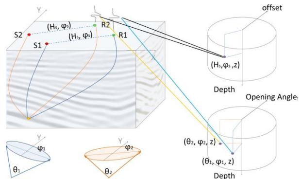
Figure 2. Two specular rays with the same offset and azimuth mapped into the same bin in the S-OVT gather but to different bins in the LAD gather
