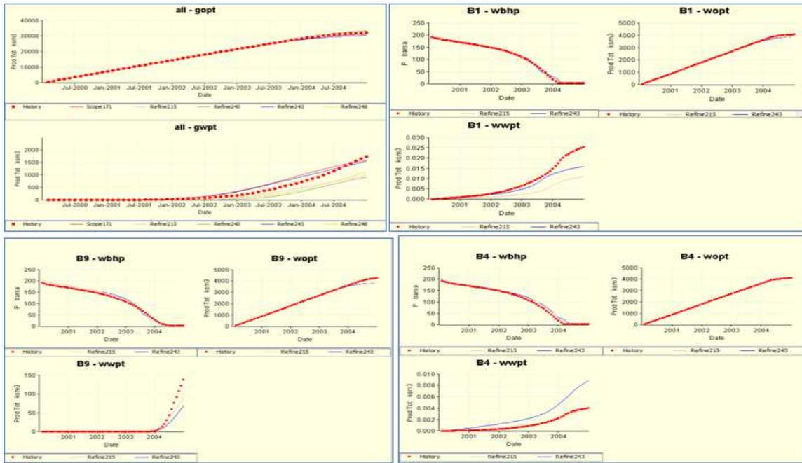
Figure-4: History Match plot for different vectors at field level and wells level
