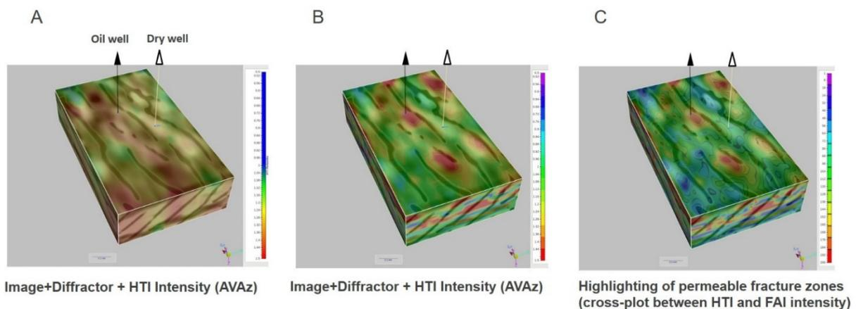
**Figure 3.** Comparison in 3D of the distribution of azimuthal anisotropy intensity (A) and FAI of the intensity of absorption of frequency (B) in SI-STs in the area surrounding the productive (black) and non-productive (yellow) well. Image (C) indicates prospective oil-saturated zones on the basis of a cross-plot between the HTI and FAI intensity attributes.
