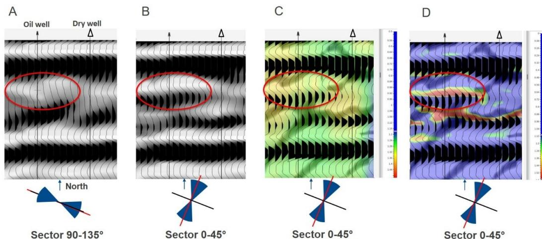
**Figure 2** Structural-tectonic oil trap of hydrocarbons in terrigenous sediments of J2 age – the longitudinal section passes through the oil-saturated and dry wells. A - depth image for the azimuth sector 90-135°; B - depth image for the azimuth sector 0-45°; C - joint depth image and diffraction
