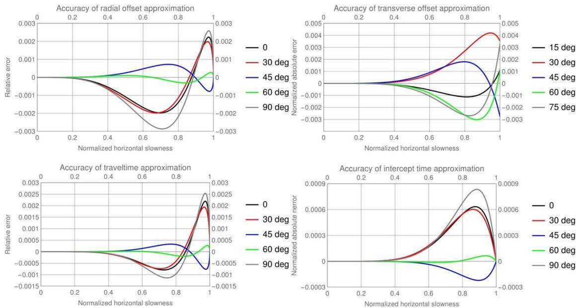
**Figure 2** Accuracy of the approximations for traveltimes, intercept time and two offset components, for different slowness azimuths. Error is plotted vs. normalized horizontal slowness  $\bar{p}_h$ .
