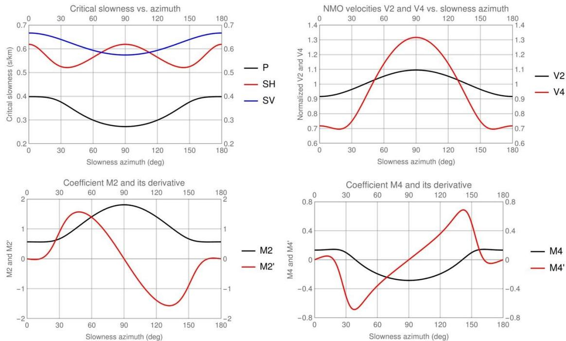
**Figure 1** Critical slowness vs. azimuth. Expansion coefficients of the vertical slowness surface for the normal-incidence and critical rays.
