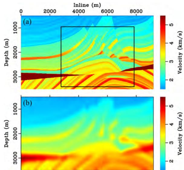
Figure 1: (a) Velocity model. (b) Smoothed velocity model obtained by using a smoothing length of 200 meters in both directions. Water body (from surface down to 500 m) is not shown. The velocity in water is 1.5 km/s.
