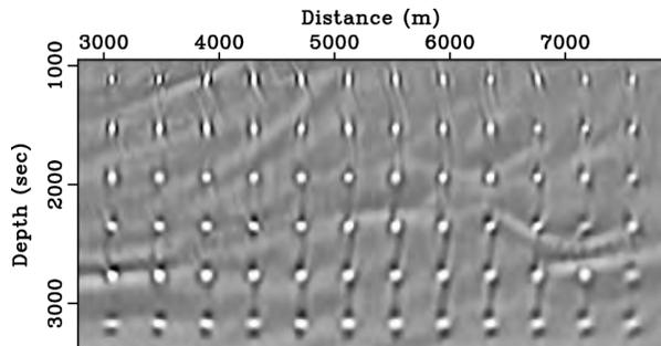
Figure 2: PSFs in the rectangular area highlighted in Figure 1(a). The PSFs are calculated from the smoothed model in Figure 1(b).
