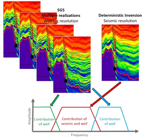
Figure 2: Modified Stochastic Inversion (MSI) analyzed in the frequency domain.
