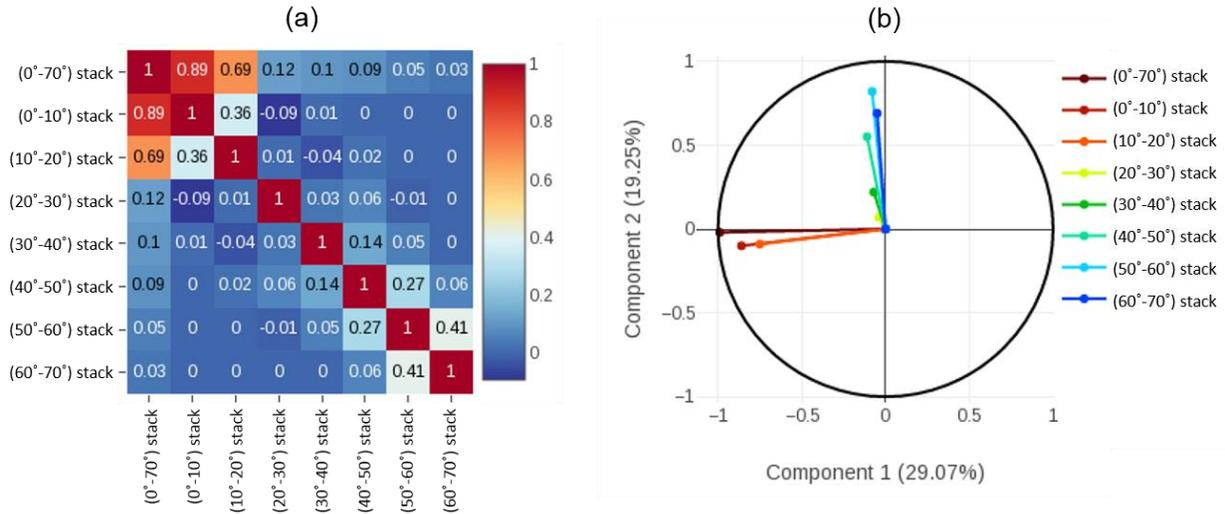
Figure 3: Eagle Ford shale data example. (a) The covariance matrix of the input dip-angle stacks. (b) Back-projecting the dip-angle stacks on the principal axes by the Eigenvectors. A projection slice is shown with respect to the first two PCs.
