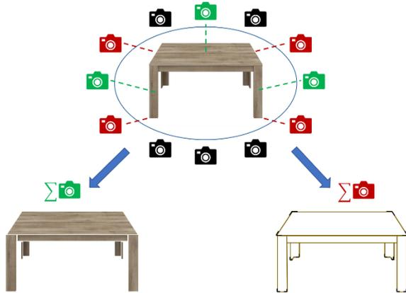
Figure 1: Distributing cameras around a coffee table object to compose its 3D image. A linear combination of direction-dependent snapshots produces a picture of the table's surfaces only (green snapshots) and a picture of the table's corners and edges only (red snapshots).
