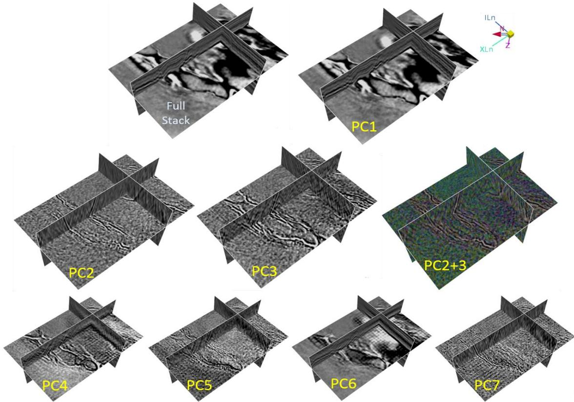
Figure 4: Back-projecting the dip-angle stacks on the principal axes by the Eigenvectors produces the PC images (numbered). The dip-angle full stack is shown for reference. Useful structural specifications may be obtained by co-rendering multiple PC images.
