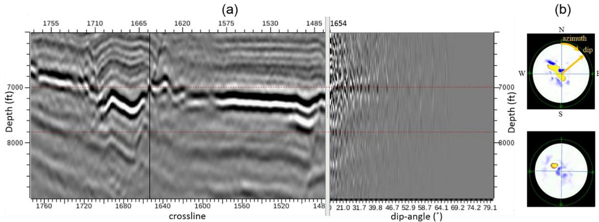
Figure 2: Eagle Ford shale data example. (a) An image stack to the left of a full-azimuth dip-angle image gather, extracted at the marked in black location. The red horizontal marks intersect a fault plane (depth 7000 ft) and a dipping-reflector (depth 7800 ft) at the gather's location. (b) At these depths, the dip-angle image gather is decomposed into polar plots showing the dip-angle signatures of the fault (top) and the reflector (bottom).
