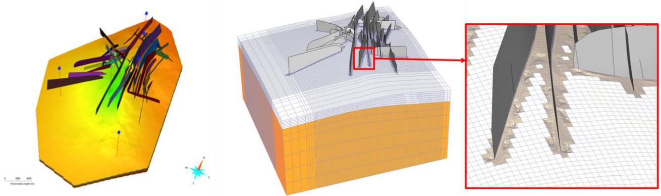
**Figure 1** Non-simplified fault surfaces integrated in a 3D structural model (left) and preserved in an unstructured grid optimized for geomechanical simulations (right).
