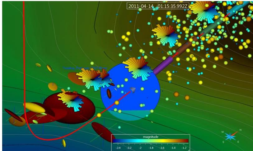
**Figure 2** Analysis of recorded microseismicity induced by stimulation operations in an EGS well, through a time-animated 3D view, including injection rate information and geological map.
