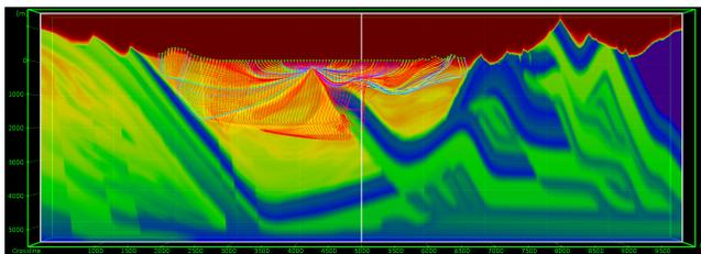
Ray tracing simulating diving waves used for refraction tomography
