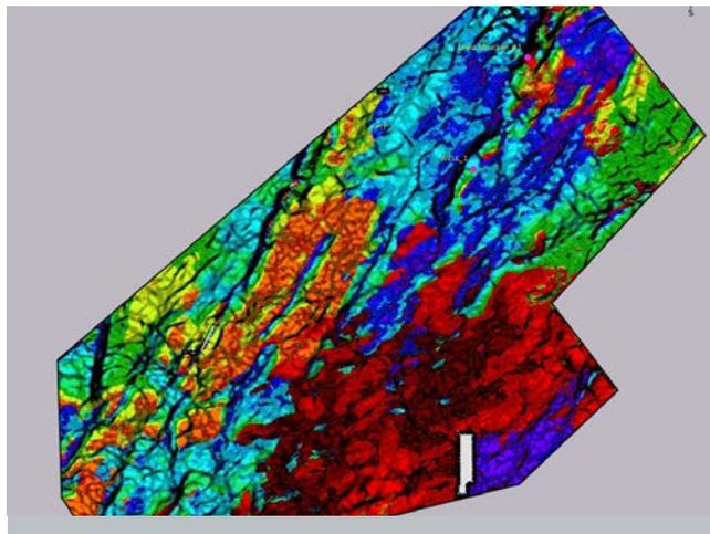
▲ Seismic facies classification based on trace shape with seismic curvature. Data courtesy of Seitel.
