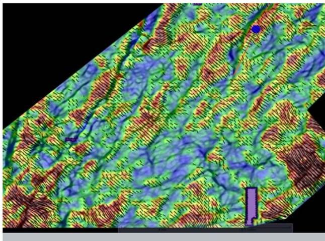
▲ Fracture and stress vectors from full-azimuth AVA(Z) inversion superimposed on curvature seismic attribute. Data courtesy of Seitel.
