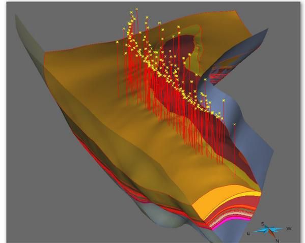
▲ Final structural and stratigraphic geological model, and current producing wells
