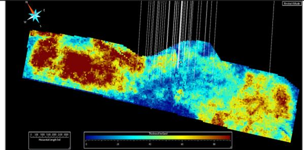
Thickness map of just one reservoir lithology, fine sand, with strong presence away from the wells. In the main structure the thickness of this lithology is around 50m in produced wells.
