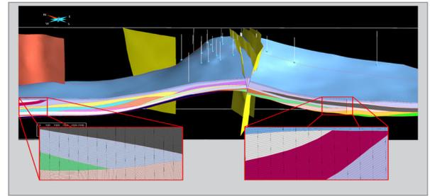
Figure 3. Geologic grid built of 24 horizon interpretations. Close up of strata terminations such as onlap, downlap and erosional truncations.
