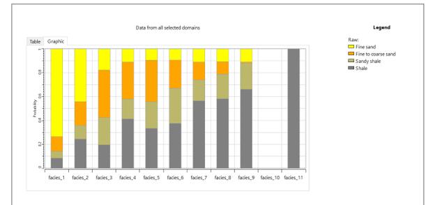
Figure 4: Calibration chart showing the presence of each electrofacies inside the seismic facies.
