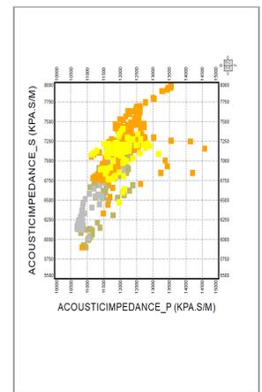
Figure 2. Crossplot between impedance logs of one well colored by facies described on core data of Lajas Formation. Cut off impedance values for each facies are not clear.
