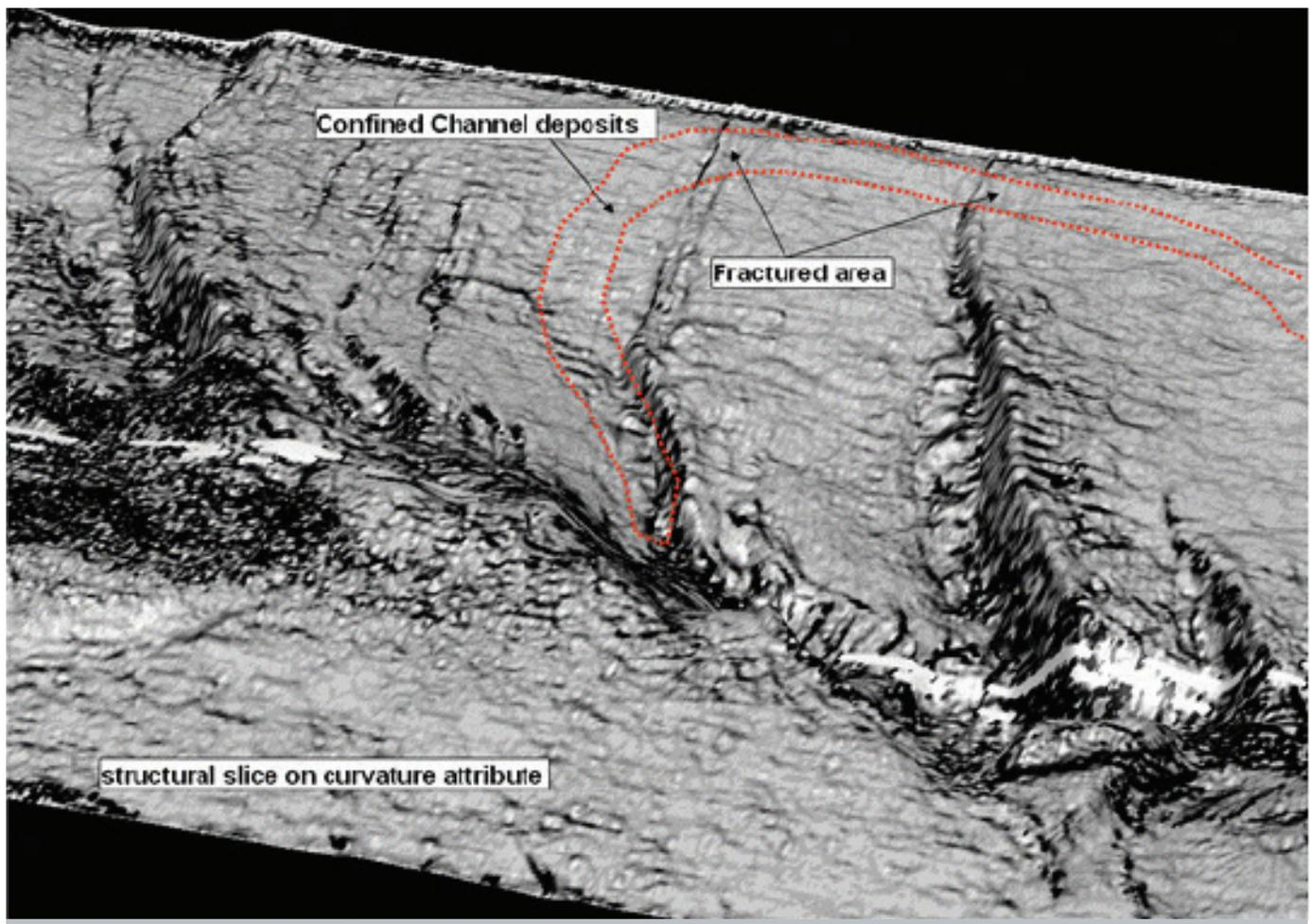
▲ Fracture area illuminated by the minimum principal curvature; structural slice on minimum curvature.
